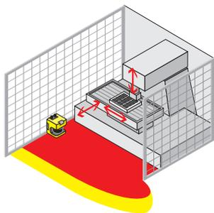
In this monitored area, different warning and protection fields can be defined by means of the software.
