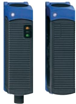
The electronic monitoring of moving safety guards including actuation in non-contact solenoid interlocks enables the wear-free and non-contact detection of the respective actuator. The patented pulse-echo technology permits large tolerances in the approach of the coded actuator, both in the switching distance and the misalignment.
