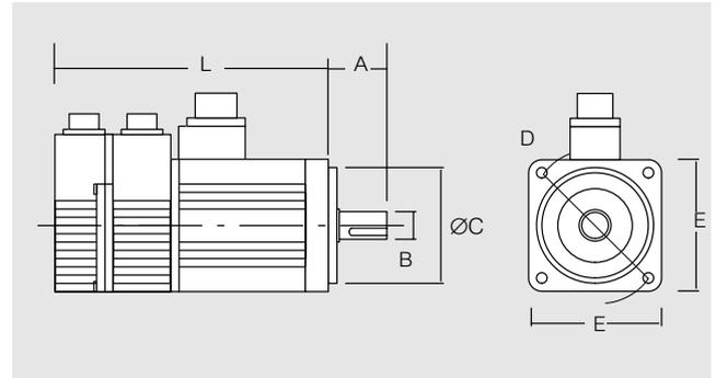
**Servomotors, 3000 rpm, cylindrical design (with brake), 400 V**
