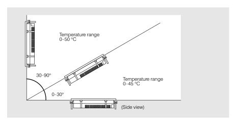
**Operating Conditions**Operation and storage depend on ambient temperature and humidity.
