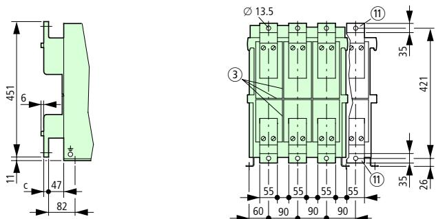
Front connection (double hole fitting) to DIN 43673: IZM1-XATF...
