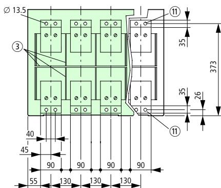
Front connection (double hole fitting): IZM2-XATF...-AV
