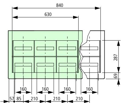
(3) Grooves (4 mm wide, 5 mm depth) for support of phase barriers in the unit
