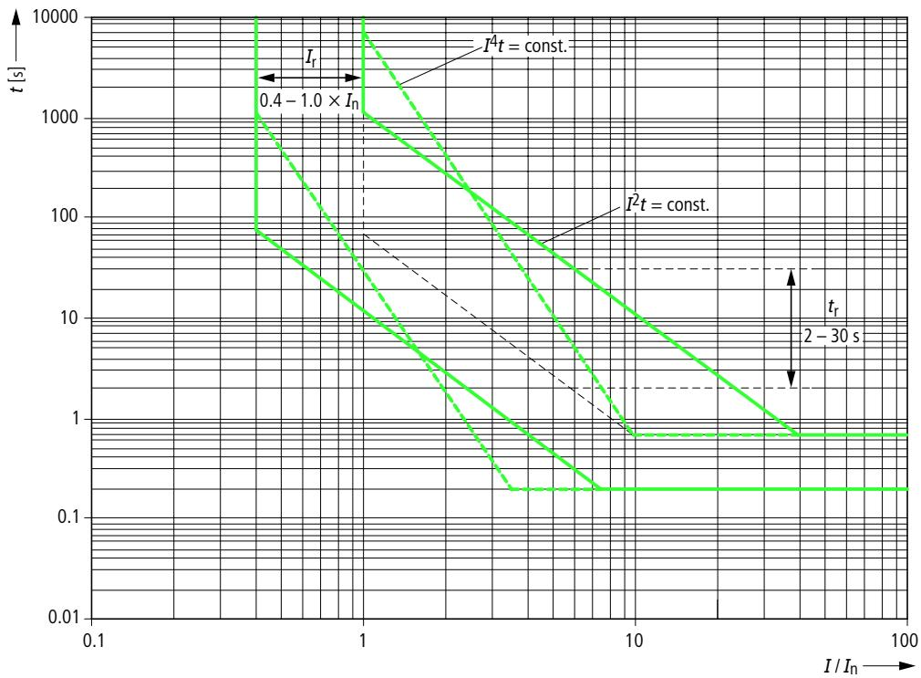
**S-trip**      ( $S$  = short-time delayed short-circuit release)
