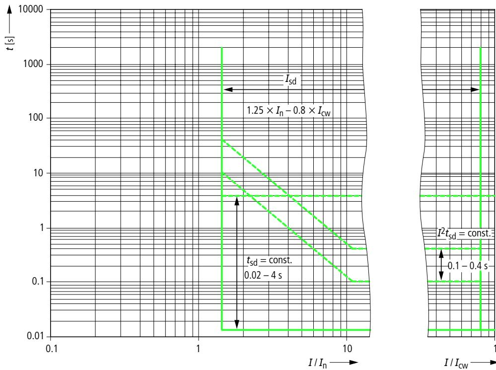
The characteristics apply for a IZMH2-... circuit-breaker, 440 V, with ground-fault protection module.
