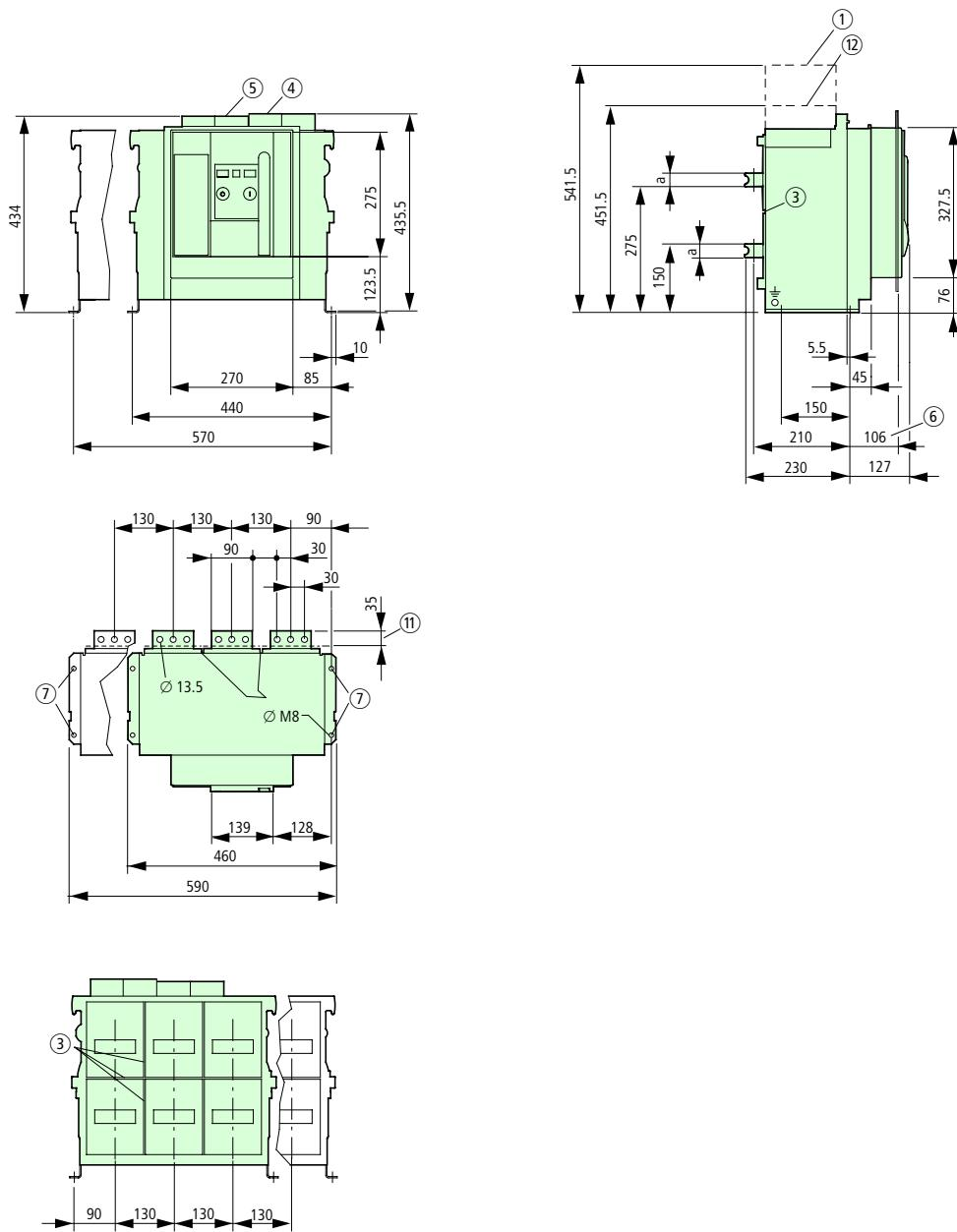
① Mounting area for removal of the arcing chambers
