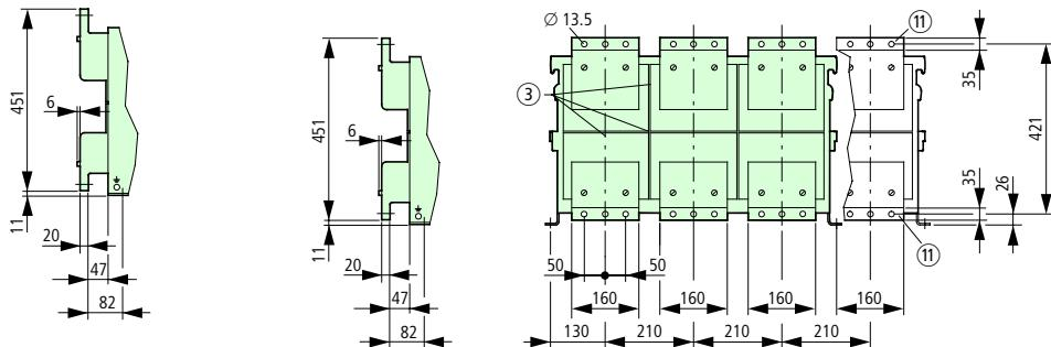
Front connection (double hole fitting): IZM3-XATF...  $\leq 4000 \text{ A}$
