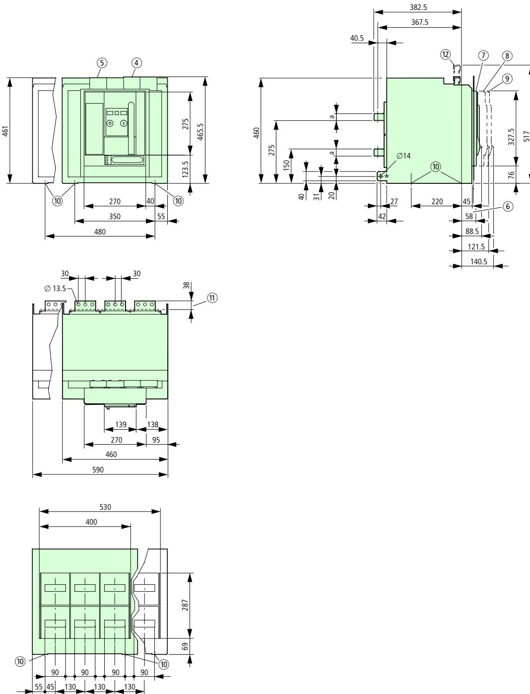
③ Grooves (4 mm wide, 5 mm depth) for support of phase barriers in the unit
