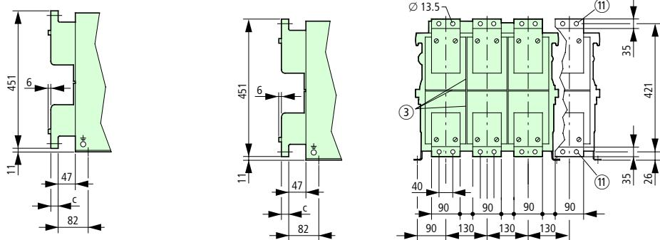
Front connection (double hole fitting): IZM2-XATF...
