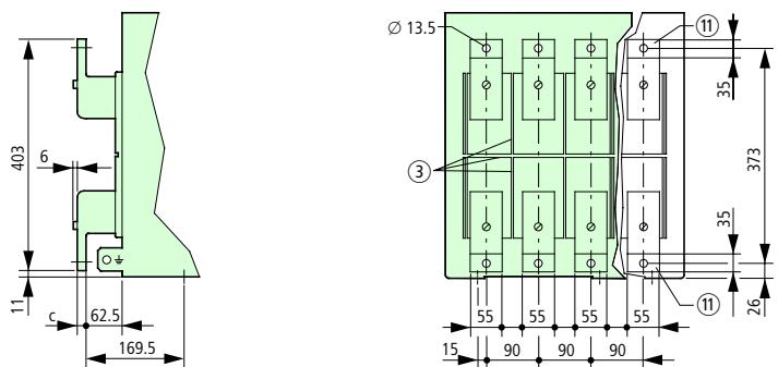
Front connection (double hole fitting) to DIN 43673: IZM1-XATF...-AV
