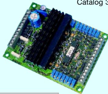
ELECTRONIC CONTROL UNIT ES/43 Serves for control of proportional valves Catalog 3/502
