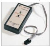
Designed to test the actuator trip unit combinations the device is plugged into the test jack on the trip unit front face. Just remove the test jack cover, insert and plug in the test device.
