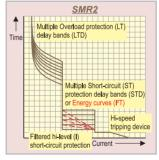
A trip unit designed to offer a overload (LT) and short-circuit protection (ST). The overload protection is adjustable from 0.4 to 1 x the chosen rating and has multiple protection bands (LTD). The short-circuit protection (ST) is
