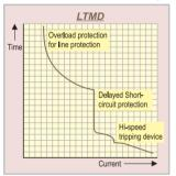
This trip unit offers overload and short-circuit protection. The overload protection is adjustable from 0.8 to 1 x the chosen rating whilst the short-circuit protection is set at 10 x the chosen rating (FD frame) or adjustable from 5 to
