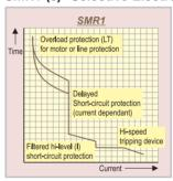
A trip unit designed to offer a overload (LT) and short-circuit protection (ST). The overload protection is adjustable from 0.4 to 1 x the chosen rating and has two protection bands (LTD), one for line protection and one for motor protection
