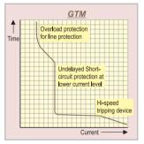
A trip unit de signed to offer overload and short-circuit protection. The overload protection is adjustable from 0.8 to 1 x the chosen rating whilst the short-circuit protection is set at about 4 x the chosen rating (FD frame) or
