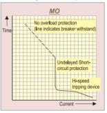
This trip unit offers short-circuit protection only, the device is adjustable from 10 to 15 x the chosen rating. In order to prevent the protection device (Circuit Breaker) from overheating, the current of the circuit that it protects, needs
