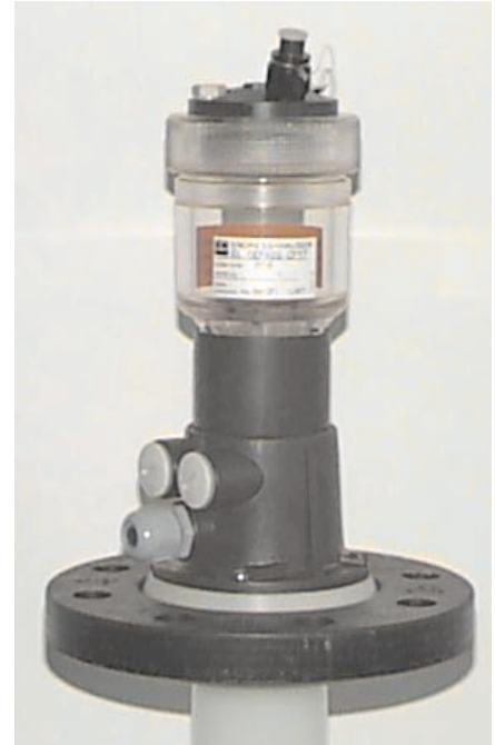
KCl reservoir mounted on top of the assembly CPA 140
